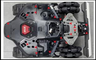
Lift up the middle frame and disconnect the marked cable, then you can take off the middle frame
