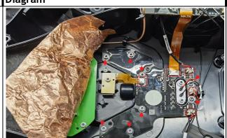
Do not forget to apply the curing glue on the connection ports that
